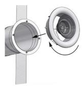
It is recommended to instal with Lindab VRGL (eventually VRGU, ILU or ILF) elements. It can be mounted directly into SPIRO pipe.
