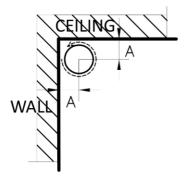
Minimum distance of "A" valve from the wall and ceiling for the pipe with a diameter:
