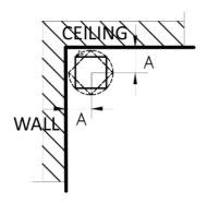
Minimum distance of "A" valve from the wall and ceiling for the pipe with a diameter:
